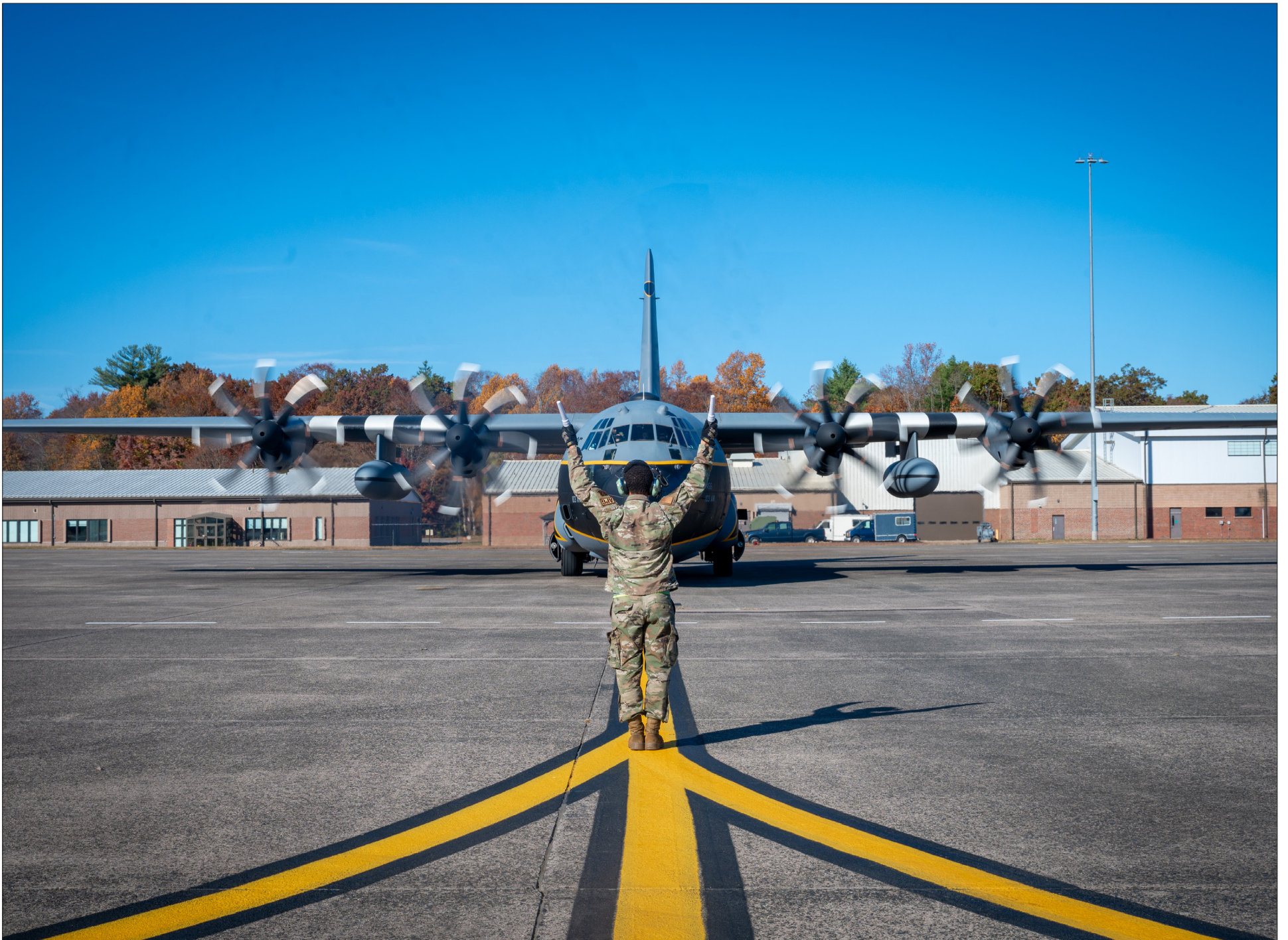
A 103rd Airlift Wing C-130H Hercules aircraft, retrofitted with new eight-blade NP2000 engines, taxis into Bradley Air National Guard Base, Oct. 25, 2024. This is the first of eight C-130s belonging to the Connecticut National Guard's Airlift Wing to be retrofitted with the new engines that will improve the aircraft's thrust, decrease maintenance time, and lower engine noise by about 20 decibels.
